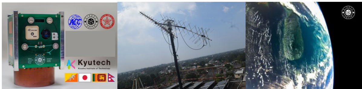
Figure 9: Left: The 1U Nanosatellite, Middle: Receiving antenna at the ground station, Right: First image of Sri Lanka taken from Space by Raavana 1 satellite. Image Credit: Annual Report (2019), Arthur C Clarke Institute.
